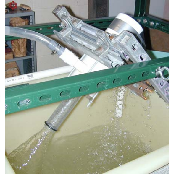
Figure 1. Side view of vortex nozzle in test stand operating at 30° inclination, with fan on left and extraction nozzle on right
