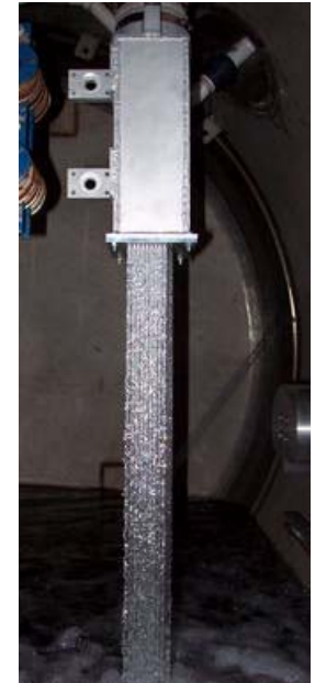
95-jet nozzle assembly in operation
