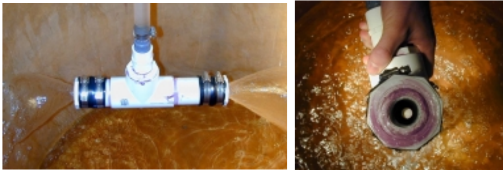
First liquid vortex created for HI-IFE shielding conditions demonstrates a smooth vortex surface and layer thickness ~50% of tube radius
