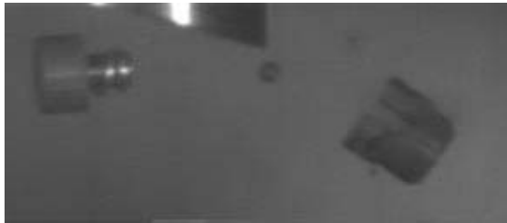
Figure 1. Sabot deflection at over 300 m/s
