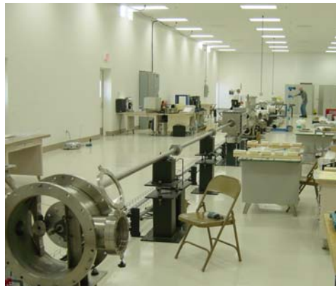
Figure 2. Target injection and tracking system is undergoing shakedown testing
