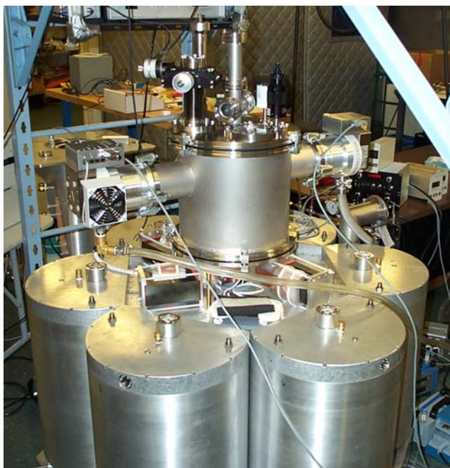
Figure 1. PLEX LLC is supplying a z-pinch based x-ray source for rep-rated materials damage studies (supported by the HAPL program)
