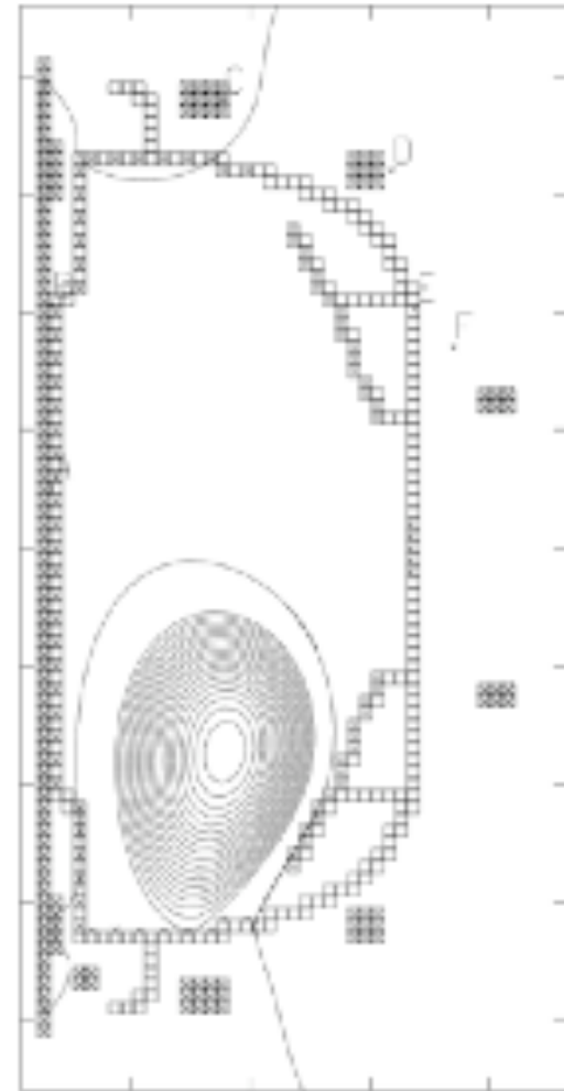
NSTX VDE, plasma is touching passive plate and divertor floor
