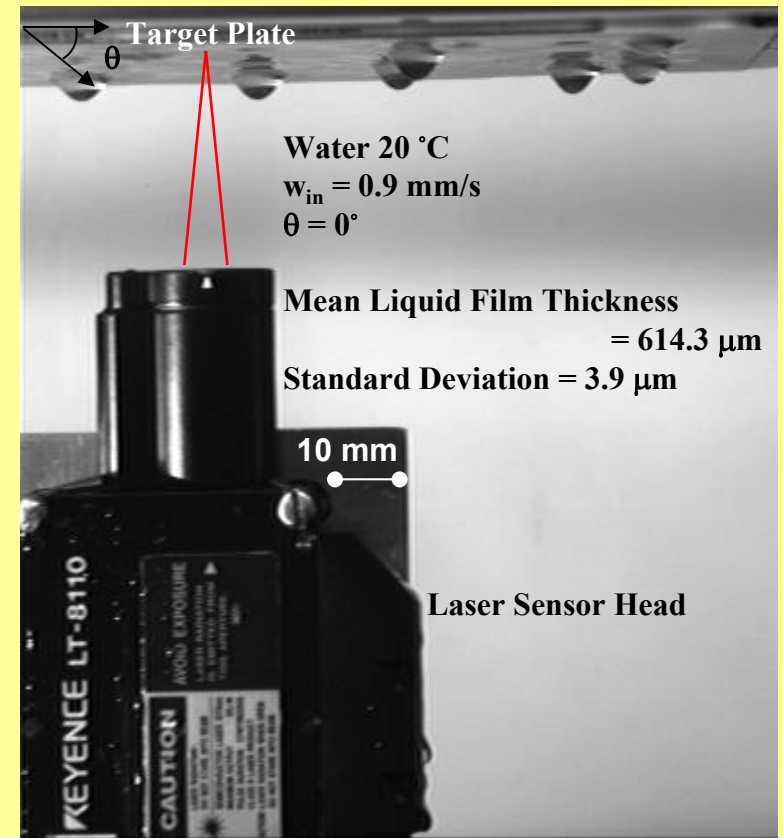
Laser Confocal Displacement Meter KEYENCE CORPORATION OF AMERICA, Model # : LT-8110
