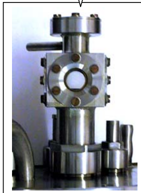
Optical test chamber
