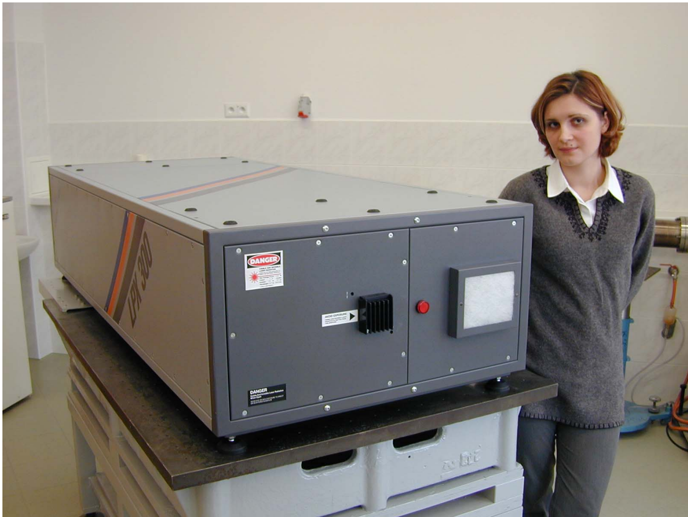
Excimer laser LPX 305i (LPX 300 series) for laser target interaction ( E_L \leq 1,2 J, wavelength 157 nm, 193 nm, 248 nm, f = 50 Hz, \tau \cong 20 ns)
