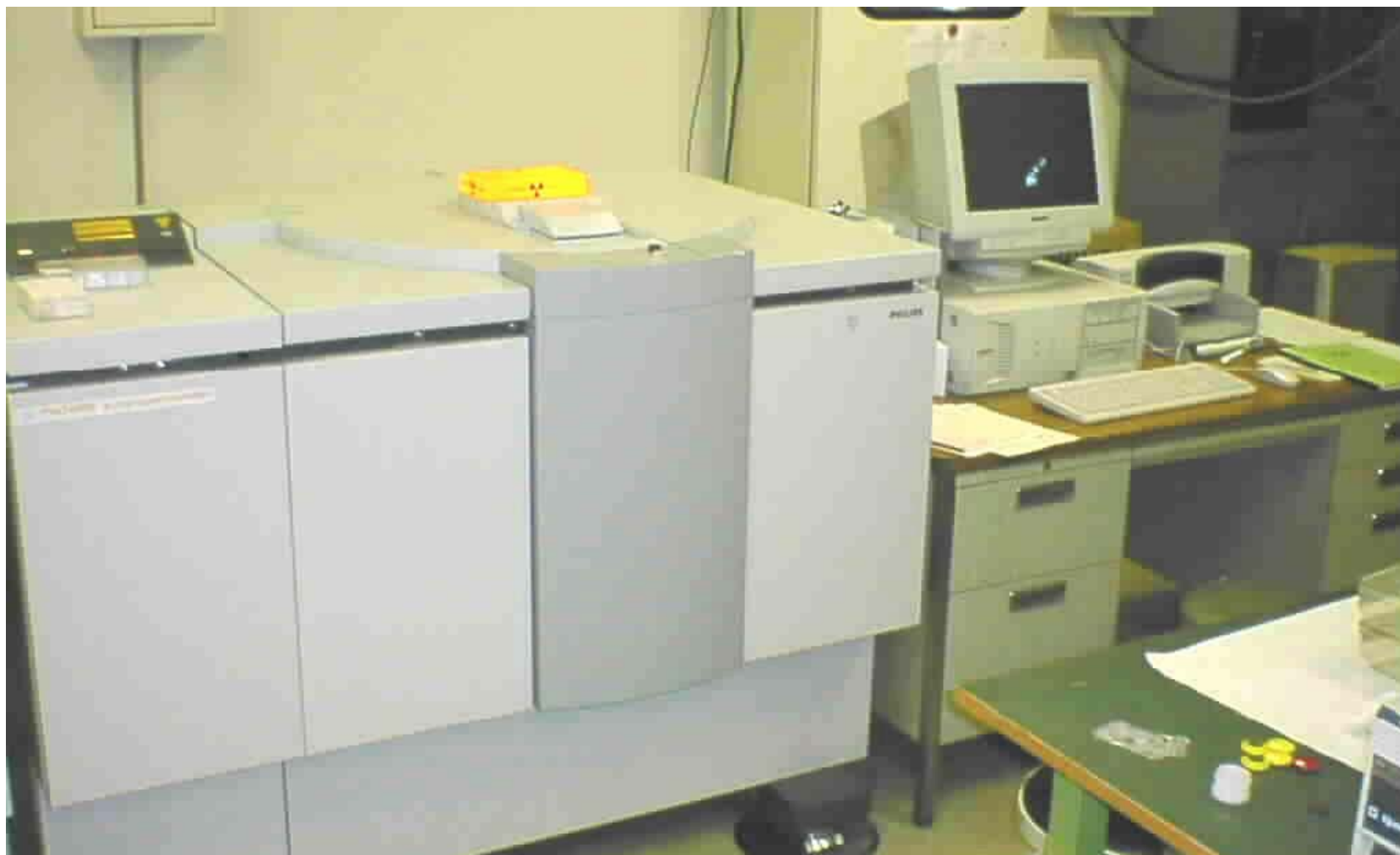
X-ray Luminescence Spectrometer for Surface Composition Analysis (Philips PW2404 System)
