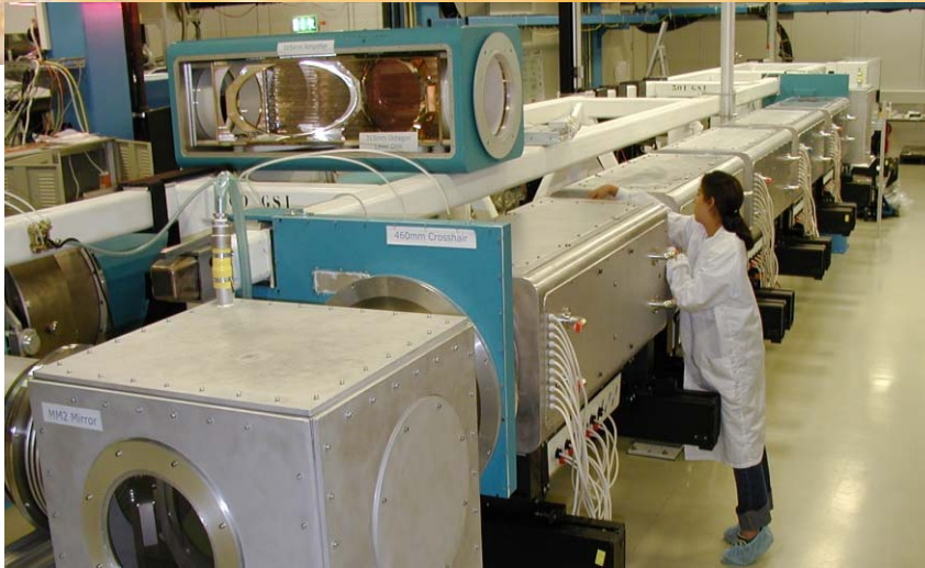
The 31.5 cm double-pass amplifier, using Nova and PHEBUS disk amplifiers, is in commissioning (1kJ in 0.5 - 10 ns)
