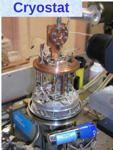
DT heater cell being installed in cryostat
