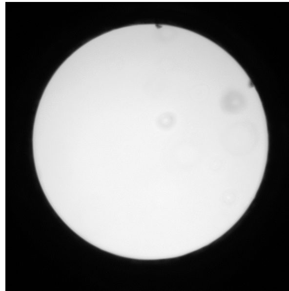
98 \mu\text{m} DT layer (total) ~50 \mu\text{m} is 'pure', while the rest resides in the foam
