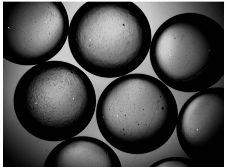
Polystyrene targets: 3 mm diameter/30 micron walls
