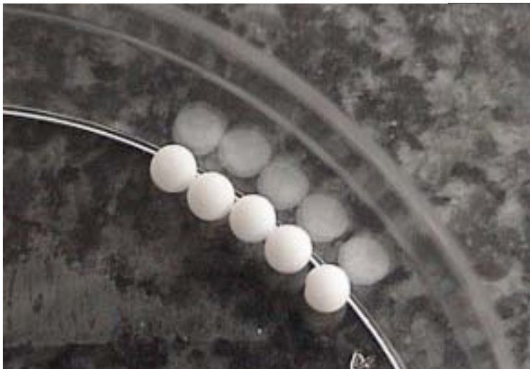
DVB shells made using microencapsulation (~ 2 mm in diameter)
