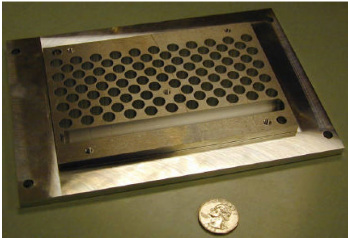
96-nozzle system uses sheet jet and multiple cylindrical jets
