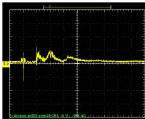
FIG. 5 Pressure trace during a flibe shot (The hydrodynamic pressure waves travelling in the chamber vanish in less than 0.5 ms. Condensation process starts at the end of the discharge ( > 2 ms) thus can be considered uniform in the volume.)
