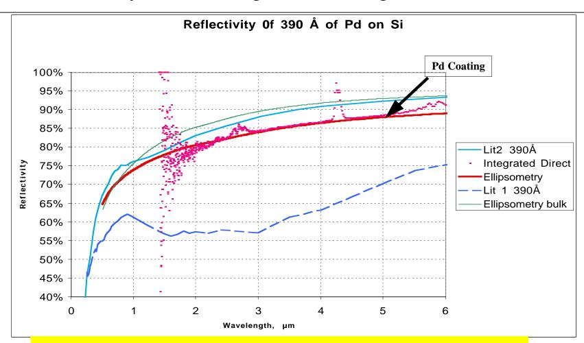
We found significant variation in literature values for Pd optical constants Fabrication and measurement methods are variable
